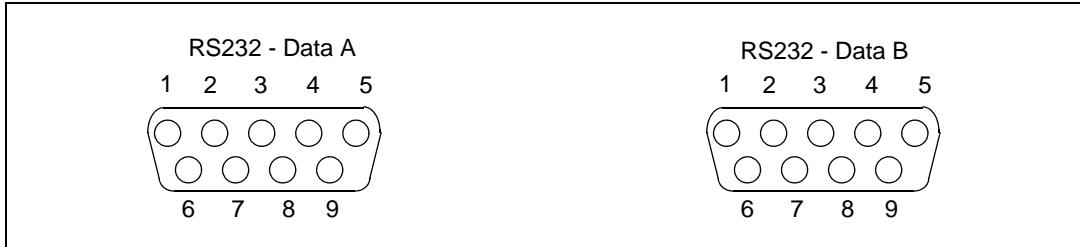
Figure 8. RS232 transmit and receive connectors: CN2, CN3
